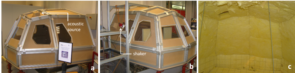
Figure 1: The cockpit mock-up : a. The acoustic source - b. The shaker on a window - c. The calibration configuration with glass wool
