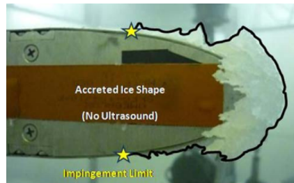
Figure 1. Ice accretion on a rotating leading edge [1].
